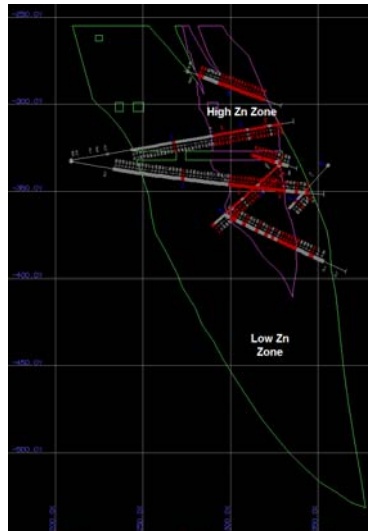
Figure 19.1: Sectional view of the two solid models – High Zinc Zone and Low Zinc Zone
